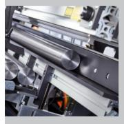
Continuous "V-Channel" for the efficient feeding of short bar sections.
