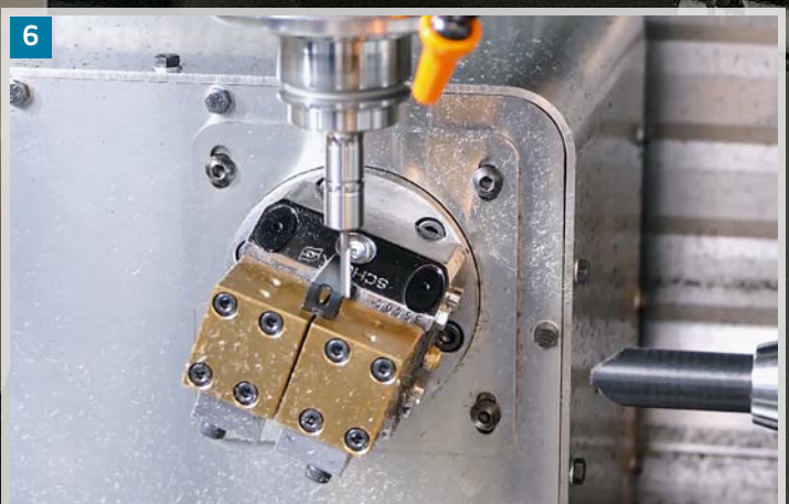
6 th face machining with the pickup unit
