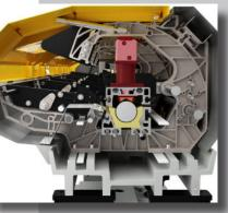
Two prisms actuated pneumatically prevent the tipping of the pusher with the holding down function of the pusher
