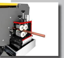
Guide steady can flexibly be converted from rollers to guide bushings (when processing polygonal material)
